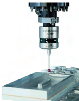
Integration between controller and sensor to measure workpiece size
