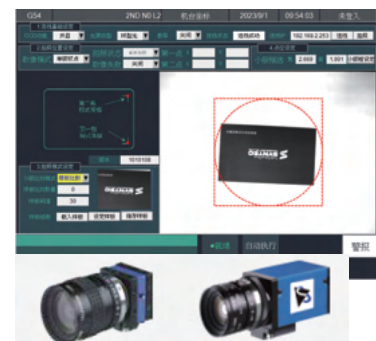
Integration between controller and vision system to compensate workpiece position
