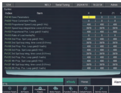
Easily adjust servo parameters by controller
